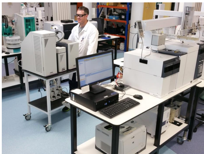
Figure 2: Refurbished analytical laboratory revealing some of the trolley enabled instruments which enable hybrid separation / detection techniques such as IC/ICPMS, LC/ICPMS, GC/QTOFMS.
