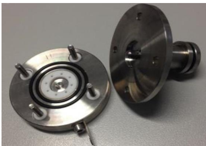
Figure 2: Split flat coin cell used to measure double layer capacitance [Oberoi A. 2015].
