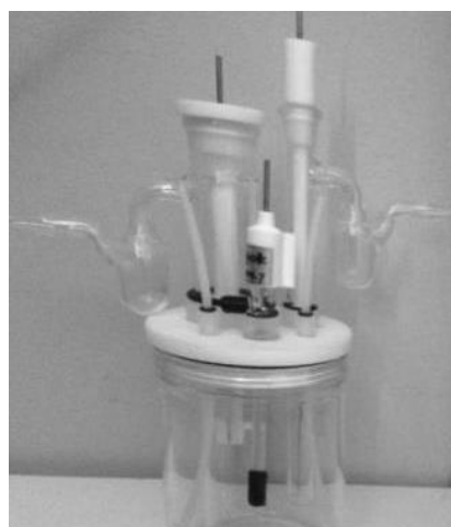
Figure 3: Three-electrode electrolytic cell used to measure hydrogen storage capacity.
