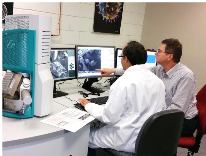
Figure 3: New scanning electron microscope with variable pressure SE detector and also fitted with an EDS package enabling elemental analysis.
